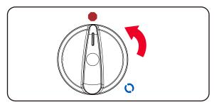
4. Turn cylinder valve to the OFF position.
