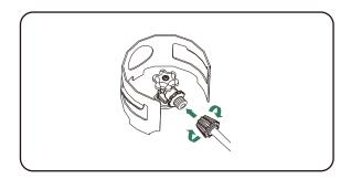
2a2. Fully open the Propane/LPG cylinder knob.
