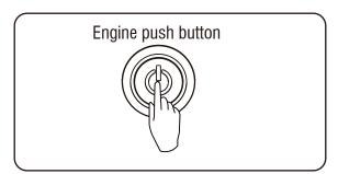
Press and hold the STOP button of the remote control fob, the engine push button red light will start flashing and then it will stay on.
