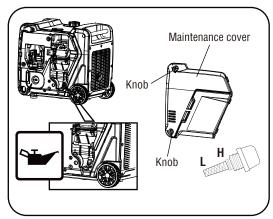
The engine is equipped with a low oil shut-off and will stop when the oil level in the crankcase falls below the threshold level.
