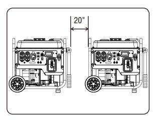
2. Both generators to be turned off and all electrical loads disconnected before paralleling operation.
