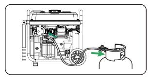
4. Open valve on propane LPG cylinder and check all connections for leaks by wetting the fittings with a solution of soap and water. Bubbles which appear or bubbles which grow indicate that a leak exists. If a leak exists at a fitting, then turn off the valve on the cylinder and tighten the fitting. Turn the valve back on and recheck the fitting with the soap and water solution. If the leak continues or if the leak is not at a fitting, then do not use the generator and contact customer service.
