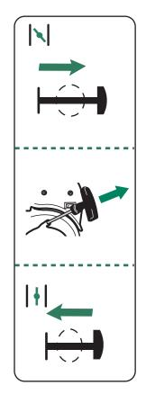
5. Start Move the choke lever to the "START" position.
