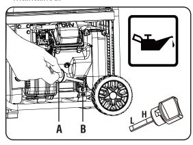
The engine is equipped with a low oil shut-off and will stop when the oil level in the crankcase falls below the threshold level.
