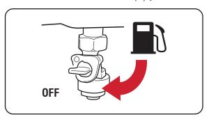
4. Turn the cylinder valve to the "OFF" position.
