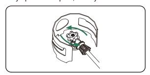
3. Turn engine switch located on control panel to RUN(I) ( ) position.
